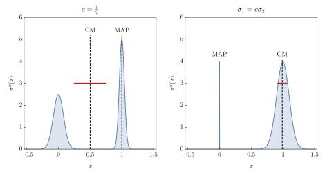
Left: the density with  $\sigma_1 = 0.08$ ,  $\sigma = 0.04$ , and  $c = \frac{1}{2}$ . The CM estimate represents the distribution poorly. Notice that when the CM gives a poor estimate, this is reflected in wider variance (1 standard deviation is depicted as a red line). Right: the density with  $\sigma_1 = 0.001$ ,  $\sigma_2 = 0.1$ , and c = 0.01. The MAP gives a poor estimate since it is in an unlikely part of the computational domain.
