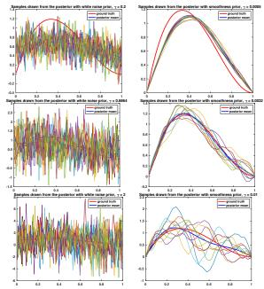
Samples drawn from the posterior corresponding to both the white noise prior and the smoothness prior for several values of  $\gamma$ . We also plot the ground truth solution and the posterior mean. The solutions in the middle row *roughly* satisfy the Morozov discrepancy principle.
